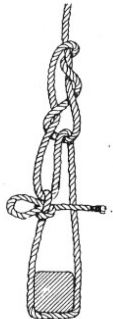
DIVER'S HITCH (FINISHED WITH A SLIPPED HALF HITCH)
